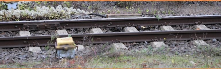
Axle counter, to keep safe distances between trains
